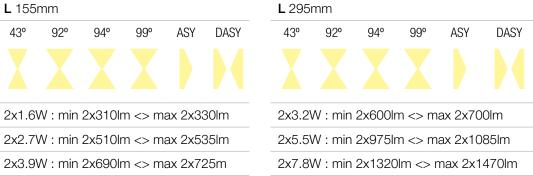
It is possible to specify individual luminous flux, beam angle and colour temperature for each luminaire side, downlight and uplight side.
